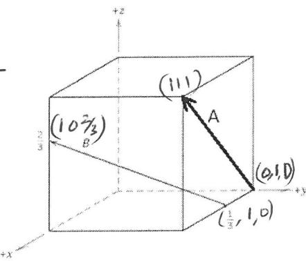
V. Determine the Miller indices for the planes (B and A) shown in the following unit cell:
