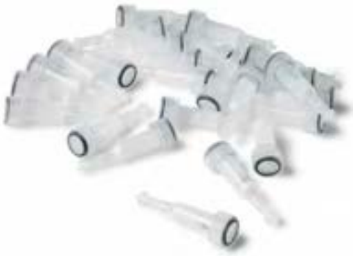
Fig. 5.6. GST SpinTrap is a single-use column for rapid, small-scale purification of GST-tagged proteins.
