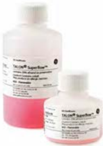
Fig 3.37. TALON Superflow allows for protein purification under native or denaturing conditions and can be used with prokaryotic and eukaryotic expression systems. TALON Superflow is available in 10 and 50 ml volumes.
