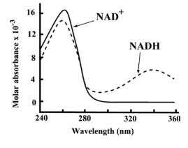
As seen here, the UV absorbance spectrum of nicotinamide is sensitive to the oxidation state. This feature is commonly exploited to monitor reaction progress of redox enzymes using NADH as a cofactor. Indeed, LDH kinetic parameters will be determined using this as our spectroscopic probe. If pyruvate, and NADH are mixed together with active LDH, NADH should be oxidized to NAD<sup>+</sup> with a corresponding decrease in Abs<sub>340</sub>.
