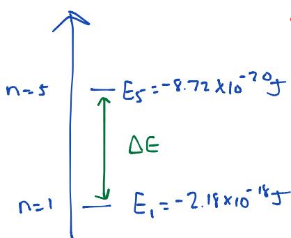
So, in the 1<sup>st</sup> shell, the  $e^-$  is attracted to the nucleus with  $-2.18 \times 10^{-18} \text{ J}$  of potential (negative is good)
