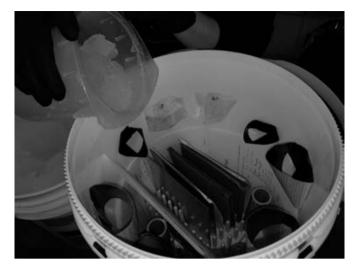
FIG. 3—Aqueous gel being placed around mock evidence arranged in a 5gal bucket. [Color figure can be viewed at wileyonlinelibrary.com]
