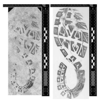
FIG. 13—*Case 007 questioned impression (left) compared to the questioned impression overlaid on a test impression from nonmated shoe 007K1 (right); note the disagreement in size. Accuracy = 97.1\% and consensus = 0.9733. [Color figure can be viewed at wileyonlinelibrary.com]*
