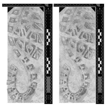
FIG. 16—Case 007 questioned impression overlaid on a test impression from nonmated shoe 007K2B with the toe aligned (left) and additionally with the heel aligned (right). Note that due to a manufacturing anomaly wherein the heel outsole was glued in a rotated but rigid position to the midsole, the two shoes' impressions cannot be overlaid, despite otherwise having the same class characteristics. [Color figure can be viewed at wileyonlinelibra ry.com]
