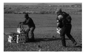
FIG. 1—Filled gel blocks may be placed around an IED to capture small shrapnel. [Color figure can be viewed at wileyonlinelibrary.com]
