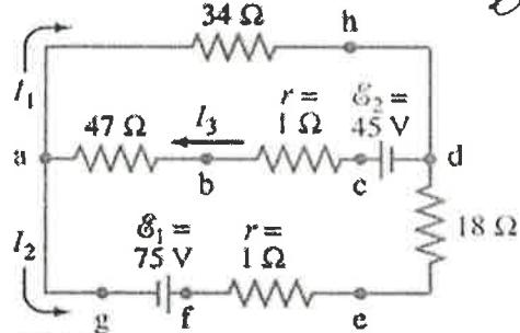
$$\text{eq } \textcircled{1} \quad I_3 = I_1 + I_2 \quad \text{junction rule } \textcircled{3}$$
