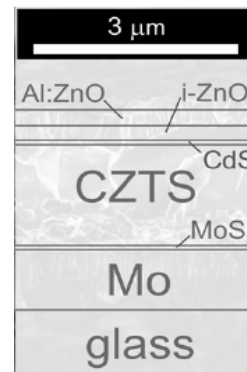
Figure 7. CZTS thin film solar cell basic device structure
